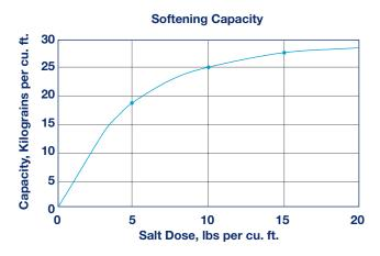
Capacity and leakage data are based on the following: 2:1 Ca:Mg ratio, 500 ppm TDS as  $CaCO_3$ , 0.2% hardness in the salt and 10% brine concentration applied co-currently through the resin over 30 minutes. No engineering downgrade has been applied.
